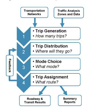
Figure B-1. The Four-Step Travel Model
